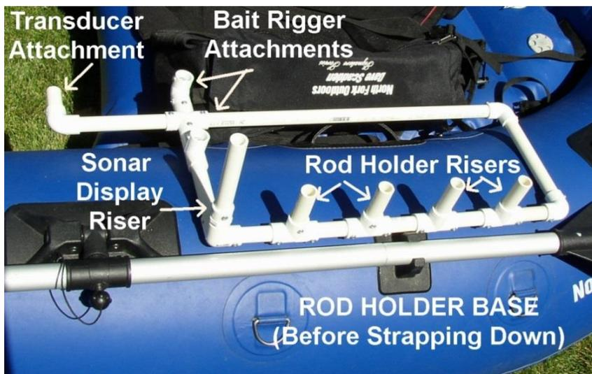
*This is my first attempt at setting up rod holders and tool racks on a Renegade. These consisted of stand-alone frames that were held in place by the strapped down pockets.*
