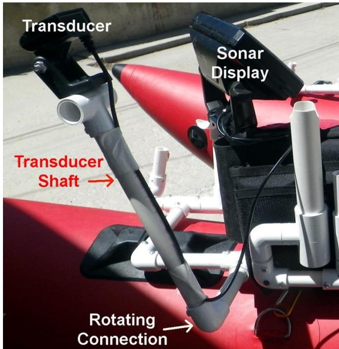
*This picture shows the sonar transducer in a full upright position. It is wise to raise the transducer while launching and beaching to avoid hard impacts on the transducer...from rocks or ramps. The sonar display is mounted so that it rides just above the left pocket. It is easily visible and may be adjusted left or right by twisting on the vertical PVC riser...up or down with the side knobs.*
