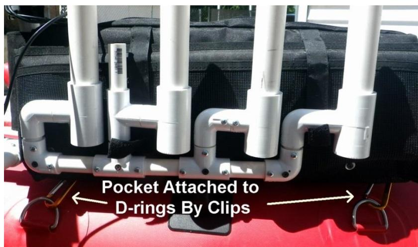
*The clips make it faster and easier to attach and remove the modified pockets. This picture shows the left side pocket, with the rod holder tubes attached. A suggestion is to make them a tight fit and then fasten them before fully inflating the air chambers.*
