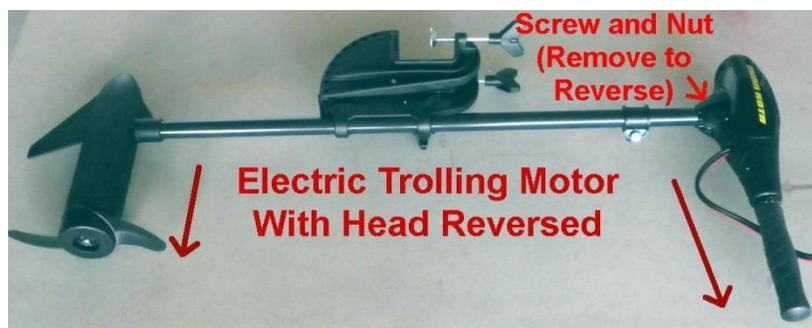
*Electric motors mounted on tubes and toons work best if they are in this configuration. The motor control head is easily rotated 180 degrees after removing the hex head bolt and nut at the base.*
