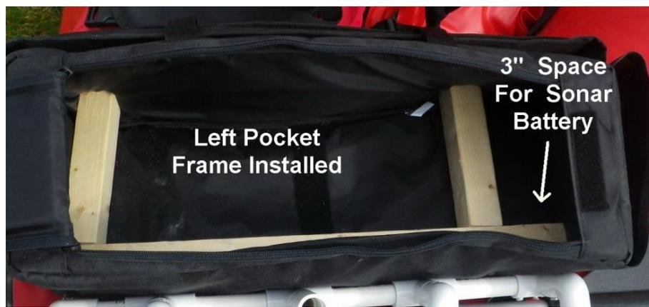
*Here is the frame for the left pocket screwed into place...including the 3" compartment for the sonar battery.*
