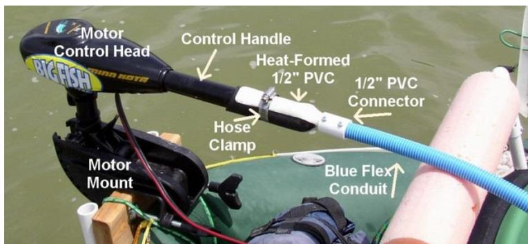
Another modification I have been making to my electric motors...for tubes and toons...is to wire in a separate ON-OFF switch between the battery and the motor. You normally use the motor control handle for on, off and speed settings. But if you get a strike while trolling or bottom bouncing it is easier and less stressful to simply flip the off switch than to try to remember which way to turn the control handle.
