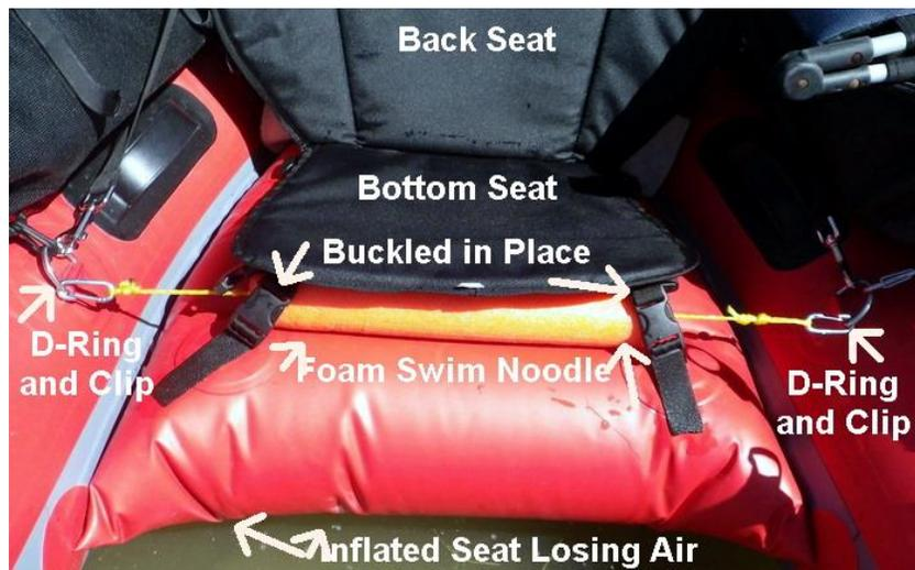
Once the butt bumper is in place you simply fasten the front buckles of the seat bottom over it to hold it in place...creating a bit of a "bucket seat" feel.
